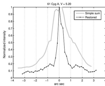
**Fig. 2.** Photometric sections of the star images 61 Cyg A, FWHM = 2.28 arc second (exposure 1 sec), FWHM = 0.65 arc second (reconstructed image).
