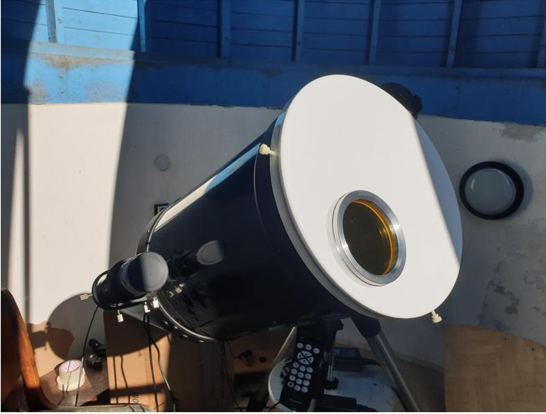
**Fig. 1.** Telescope and rejection filter used for the solar observations in AO-Belogradchik.
