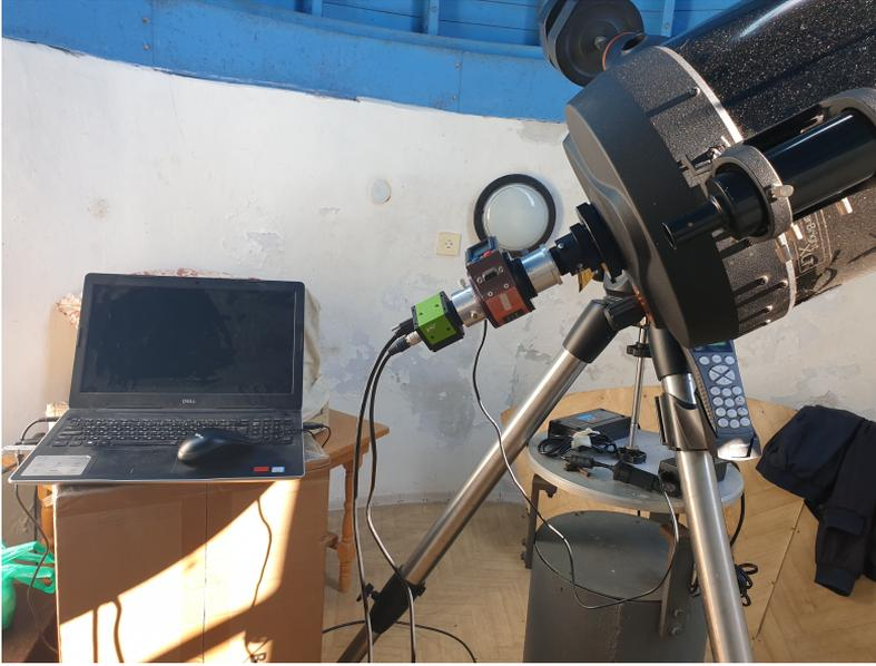
**Fig. 2.** Filter and camera system used for the solar observations in AO-Belogradchik.
