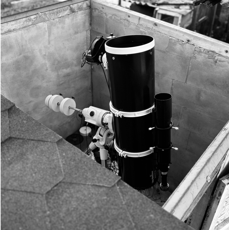
Fig. 1. The telescope at the Meshtitsa Observatory, a 0.25 m Sky-Watcher Newtonian reflector ( f/4.8 , focal length 1200 mm) mounted on an EQ6-R Pro German equatorial mount.
