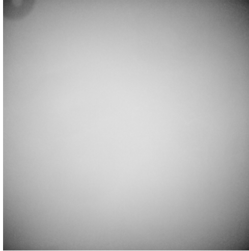
Fig. 8. Master flat field obtained in the V filter, created from the median combination of multiple twilight flats.
