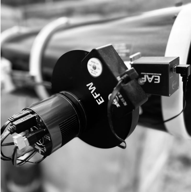
Fig. 3. Camera ASI533 MM Pro CMOS, filter wheel, and automatic focuser mounted on the 0.25-m telescope
