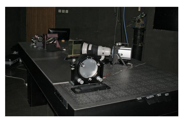
The éshelle-spectrograph is a cross-dispersed, bench-mounted, fiber-fed instrument giving a resolution from ~30000 to ~45000.
