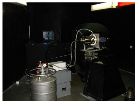
The Coudé-spectrograph allows us to obtain stellar spectra with a high resolution and "signal-to-noise" ratio of about 1000 and velocities in space with an accuracy of 500 m/s. It is equipped with ANDOR Newton 940 CCD camera (2048×512 ps, 13.5×13.5 µm).
