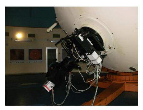
Observations with the focal reducer and in direct RC focus are carried out with ANDOR iKon-L BEX2-DD and ANDOR iKon-L E2V 42-40 CCD cameras (2048×2048 pixels, 13.5×13.5 µm size).
