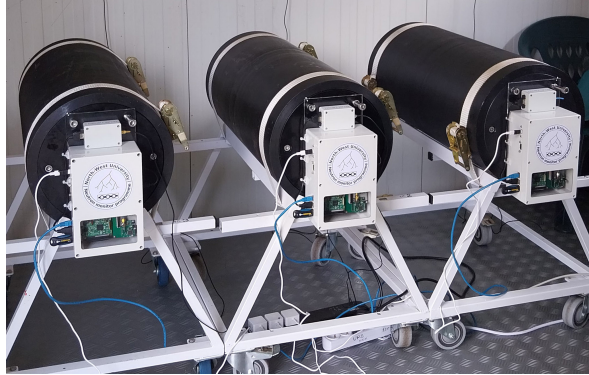
Figure 2: Completed and installed system of 3 mini-neutron counters on the territory of the National Astronomical Observatory. MNM-Rozh is currently still running in calibration mode.
