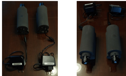
Figure 4: Visible and near-infrared (VNIR) hyperspectral imaging (HSI) sensors.
