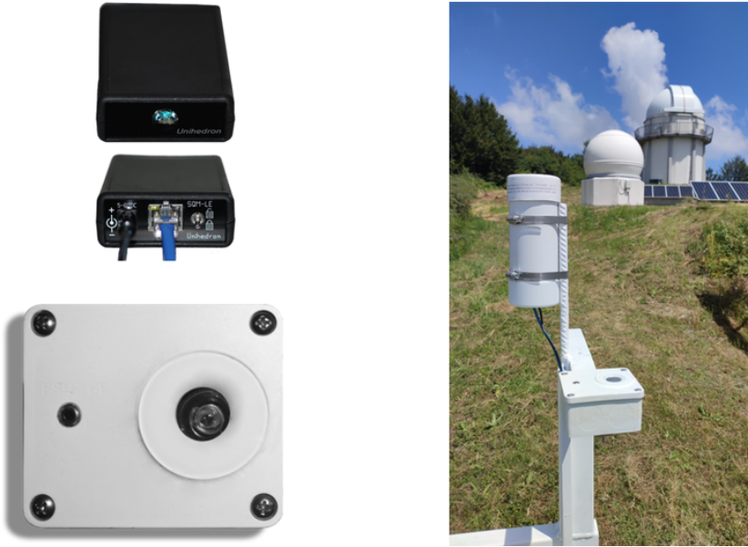
Figure 3: Sky Quality Meters (top left), TESS-W Photometers (bottom left) and both instruments mounted at Astronomical Station Vidojevica (right).
